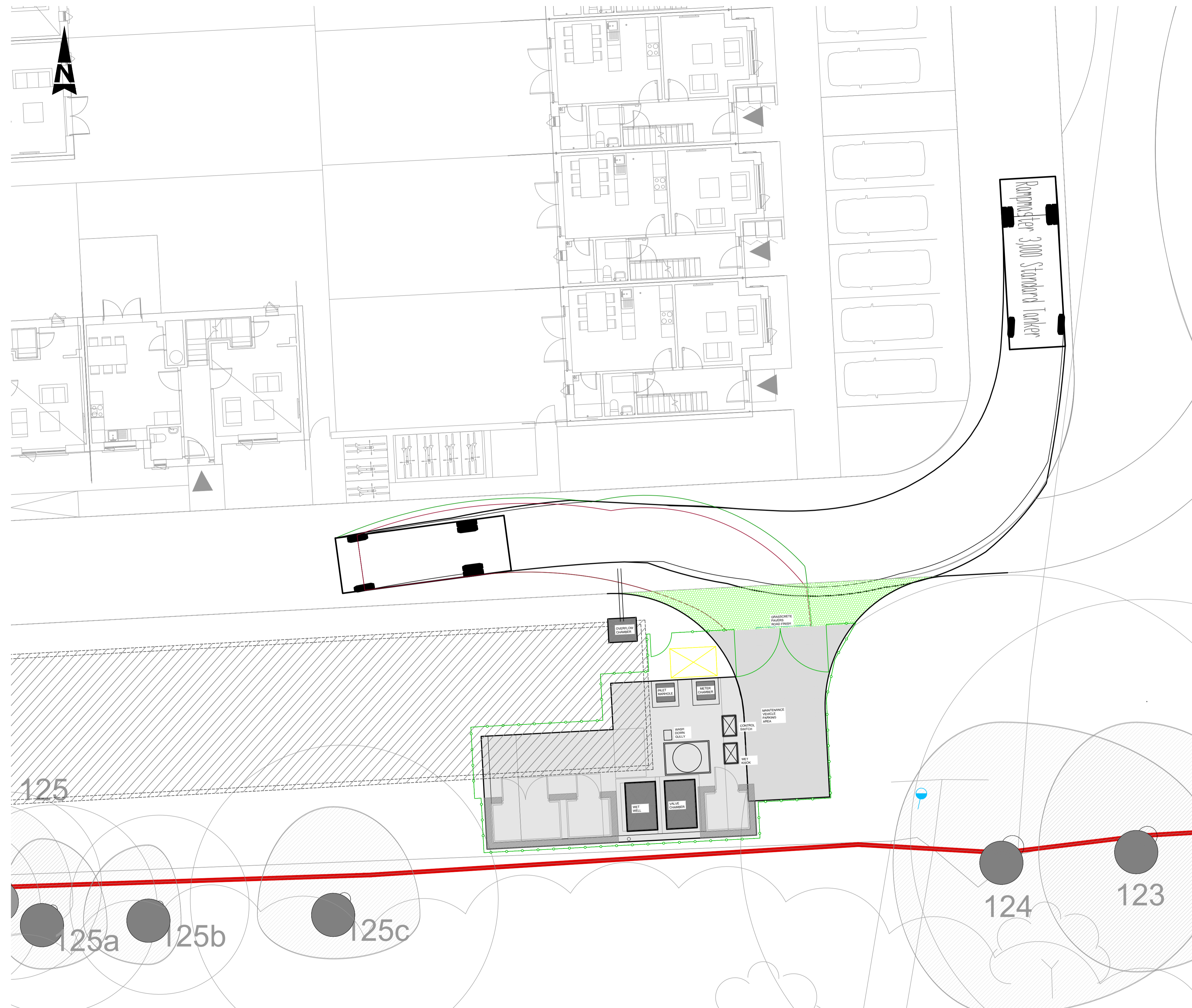
FOUL PUMPING STATION AND 24 HOUR EMERGENCY STORAGE TANK (732m3)
